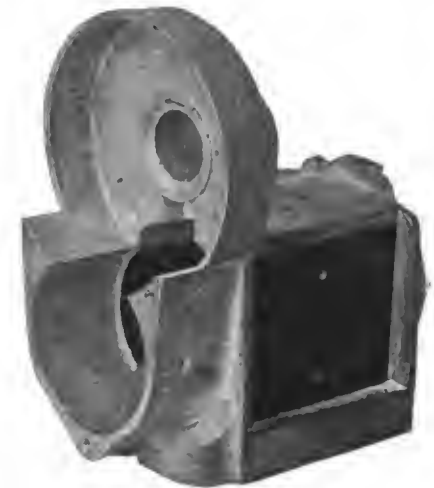
Die casting used in Eisemann magneto. The pole pieces are cast in place and hardly any machining has to be done on this whole piece, which replaces nearly twenty small parts used in the older designs.
